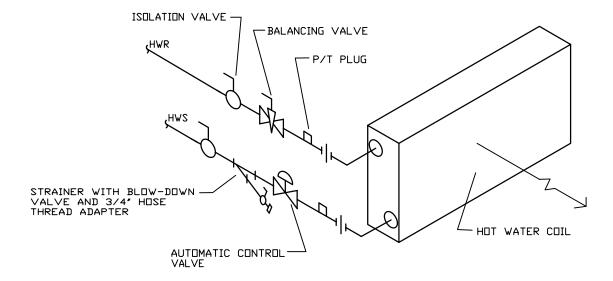
PROVIDE AIR VENTS AT COIL AND ALL HIGH POINTS OF PIPING.
